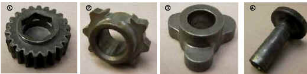
Fig.1 – Precision Forged Components Developed During the TCS Programme.
