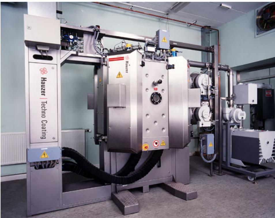
**Figure 1 - Hauser HTC 1000 – ABS advanced PVD coating machine**
