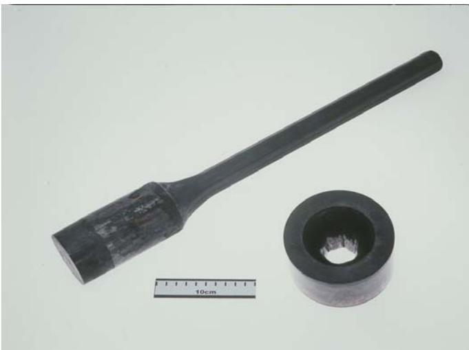
**Figure 2 A chisel bit for a pneumatic digger and extrusion die**
