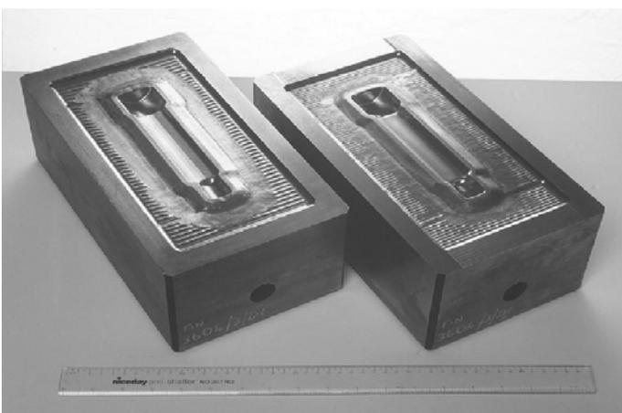
**Figure 2b Die used for precision hot forging of turbine blades for aero-engines**
