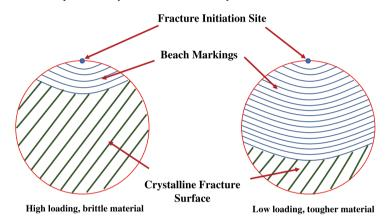
Figure One Illustration of a Typical Fatigue Failure Fracture Surface
