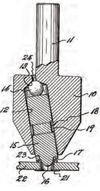
Figure 1. Bregen riveting tool (US Patent 2,739,726)
