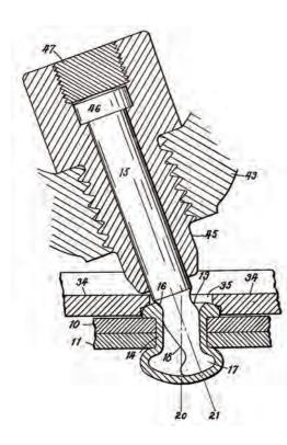
Figure 2. Deshon et. al. riveting device (US Patent 2,185,939)
